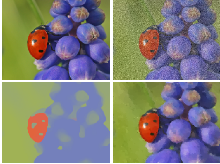
Fig. 3. Denoising of a color image I : \Omega \rightarrow \mathbb{R}^3 by separately denoising its intensity |I| \in \mathbb{R} by the usual ROF model, and chromaticity I/|I| \in \mathcal{S}^2 by the ROF model for values on \mathcal{S}^2 using the proposed method. Left to right, top to bottom: input image; added noise; denoised chromaticity; combined denoising result.
